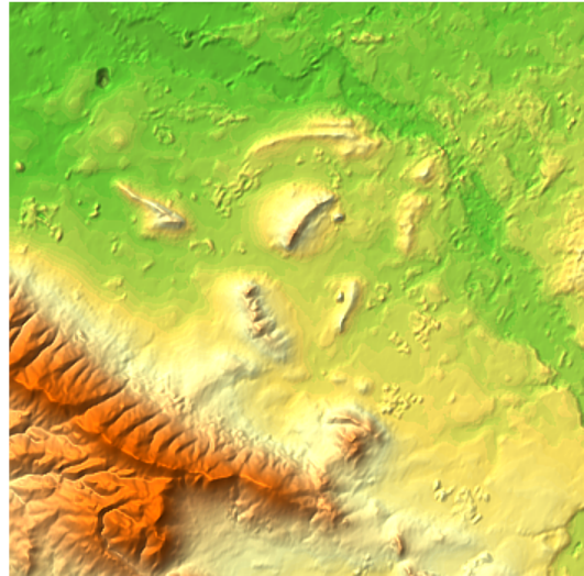
b) preprocessed DTM without Forest Canopies, noise filtered
