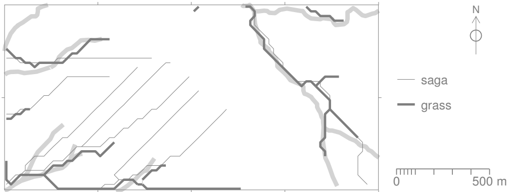
Figure 2. Hydrological networks extracted using the 1 arcsec SRTM DEM (DEMSRTM1.asc) dataset in SAGA GIS and GRASS GIS, as compared to stream network digitized from the 1:24k topo-map (grey bold lines).
